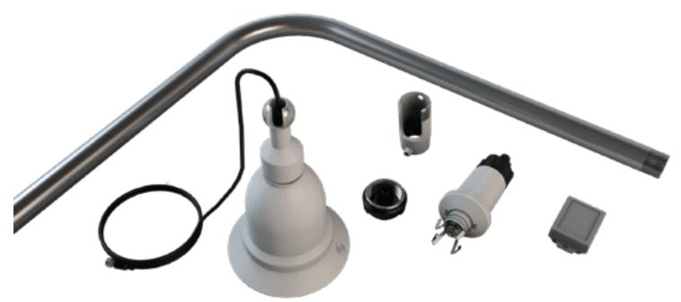
SMARTMOUNT Luminaire (LU) standardizes installations to luminaire arms and provides the ideal height while remaining within bucket truck limits and avoiding power lines. SMARTMOUNT LU includes the Bell Camera, Junction Box, GRIDSMART 3' x 3' pole, mounting components, and Electronic Protection Module (EPM).
