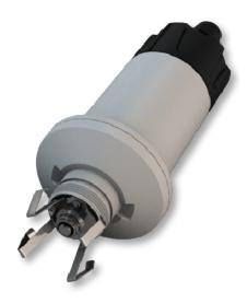
The self-grounding Junction Box offers additional surge protection for the camera while providing a Simple, easy to install, water-tight interconnection between SMARTMOUNT and the pulled CAT5e from the cabinet. The premeasured, shielded cable from SMARTMOUNT connects using a threaded M12 connector to the Junction Box. The pulled CAT5e from the cabinet connects through a cable gland for water protection and is terminated using an RJ45.
